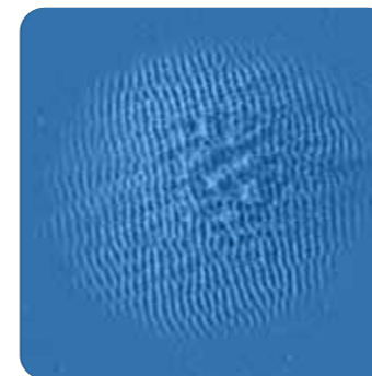
Surface functionalization with conventional system (Gaussian Beam)
